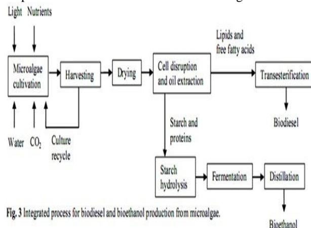
Fig. 3 Integrated process for biodiesel and bioethanol production from microalgae.
