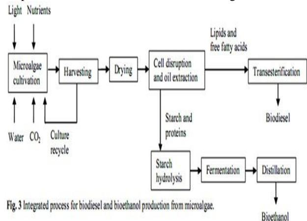
Fig. 3 Integrated process for biodiesel and bioethanol production from microalgae.
