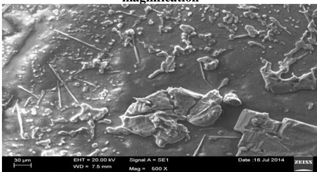
Fig 8. SEM image of optimized formulation under 500X magnification
